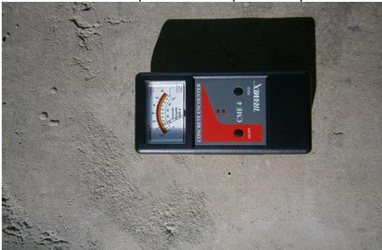
Pictured moisture reading of a Concrete Screenshot
