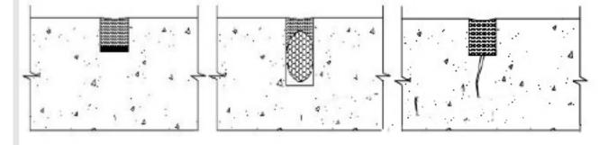
2. The backer rod supports tooling so after installation of material the sealant can be pushed to the bond line with a spatula, ensuring wet-out of the sealant to the substrate.
