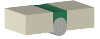
The backer rod comes in three main types, closed cell, open cell, and a hybrid that has closed outer cells but open interior cells. Each one of these types of backer rod has its own niche that it thrives in.
