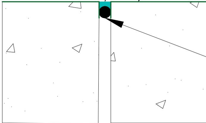
Install backing rod (or bond breaker tape), to control sealant depth,
