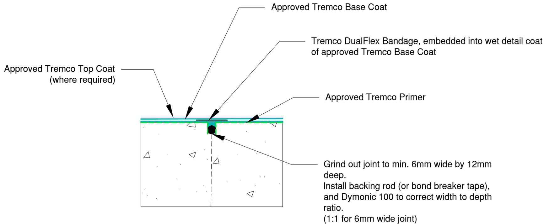
Consult Tremco for project specific advice for cracks/ joints with significant movement anticipated.
