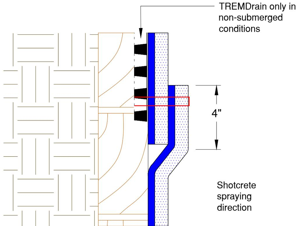
When spraying shotcrete or other materials against Paraseal LG, spray either directly at the seam or at the closed edge of the seam so as not to lodge sprayed materials between the lapped sheets. Never spray into open edge of seam.
