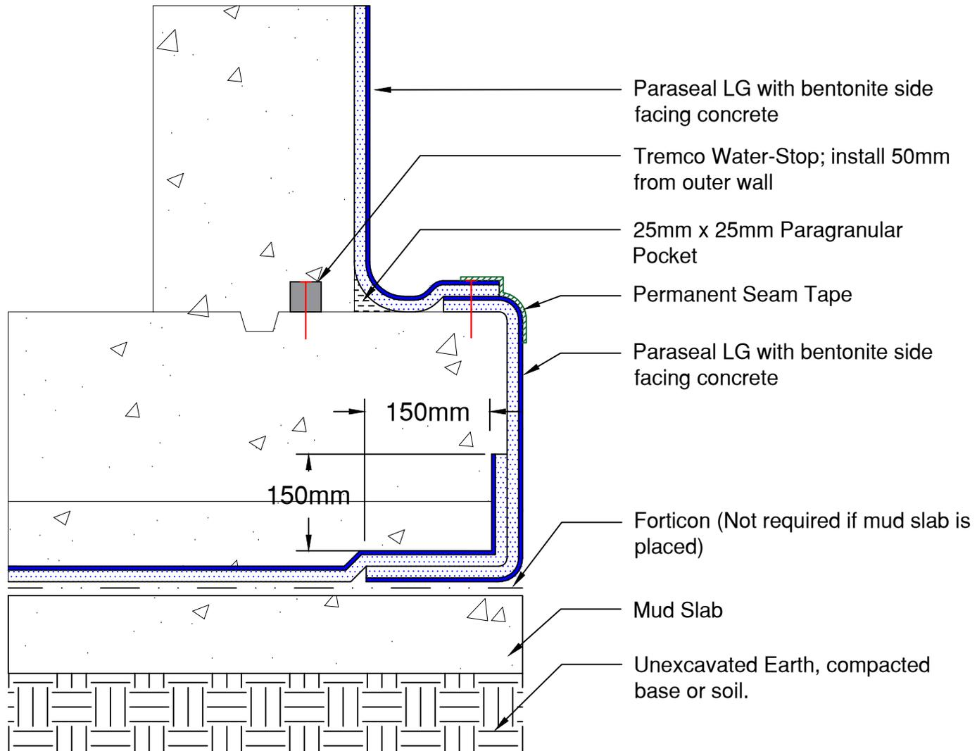
NOTE: Paraseal products require a min of 117 kg/m<sup>2</sup> of compaction/confinement in order to function as designed.
