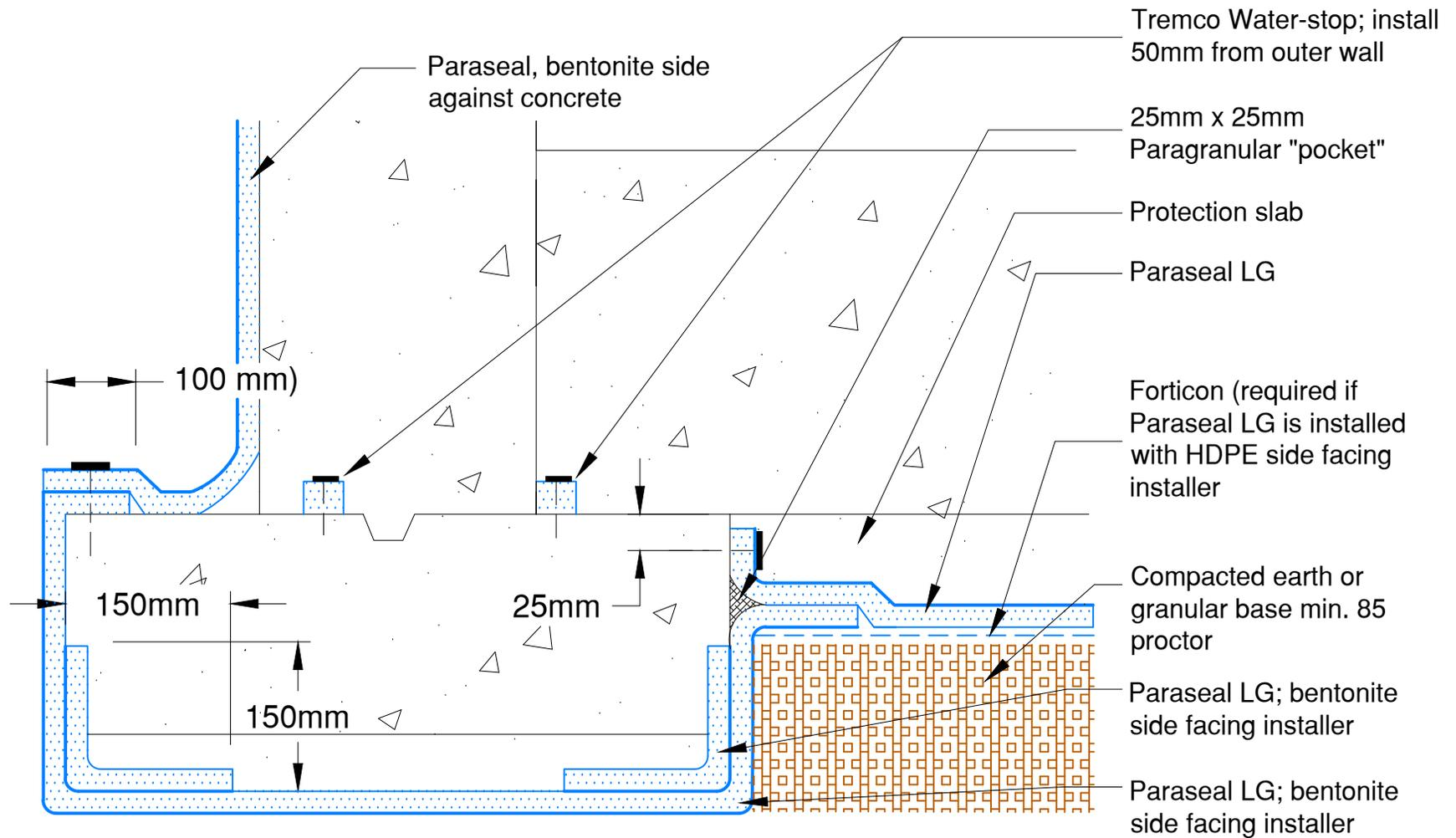
Note: Paraseal products require a minimum  $117\text{kg/m}^2$  compaction/ confinement to be effective.
