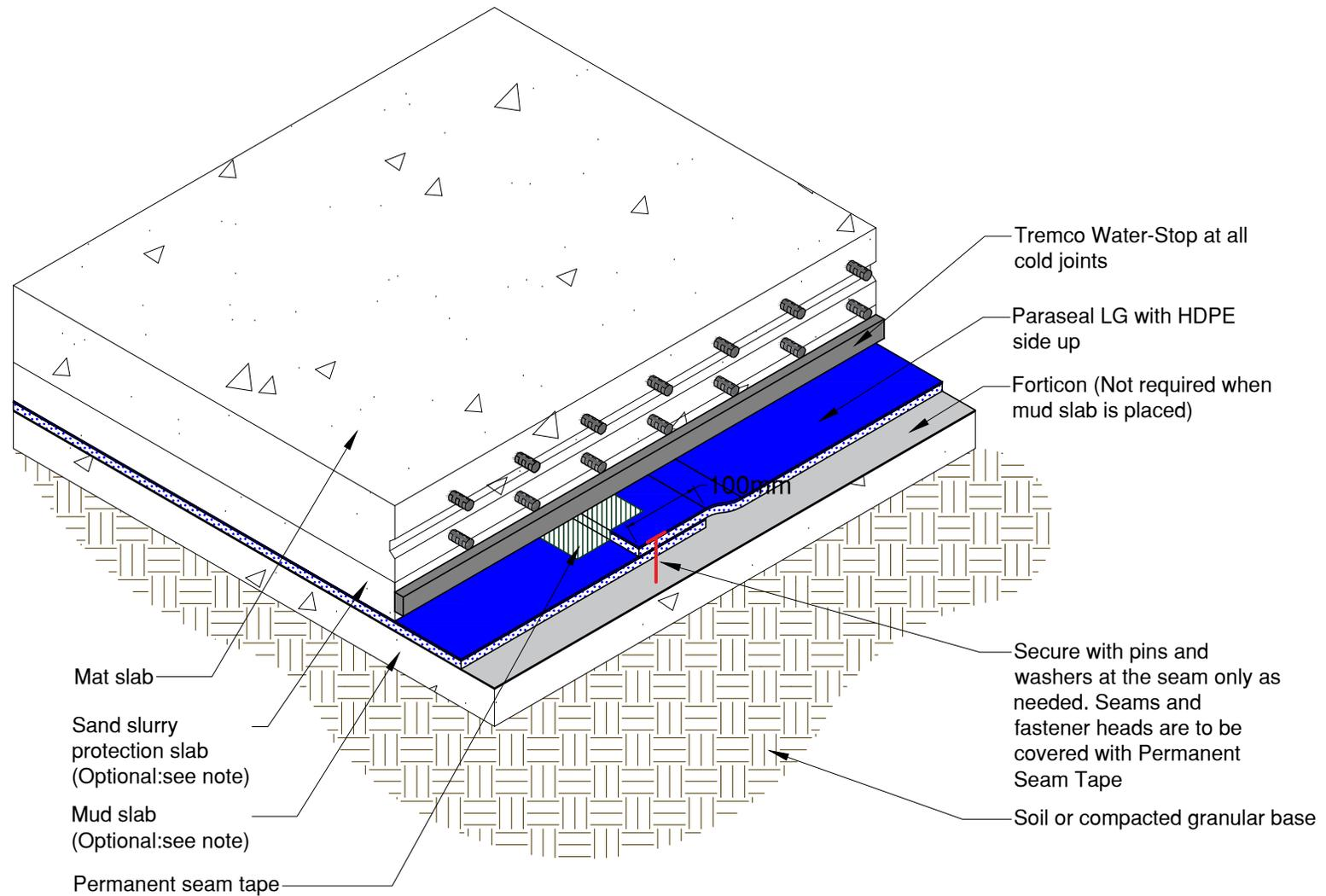
NOTE: Sand slurry protection slab and mud slab are recommended for reinforced slabs greater than 150mm thick.
