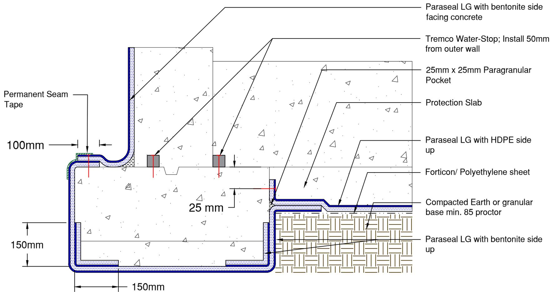
NOTE: Paraseal products require a min of 117Kg/m2 of compaction/confinement in order to function as designed.
