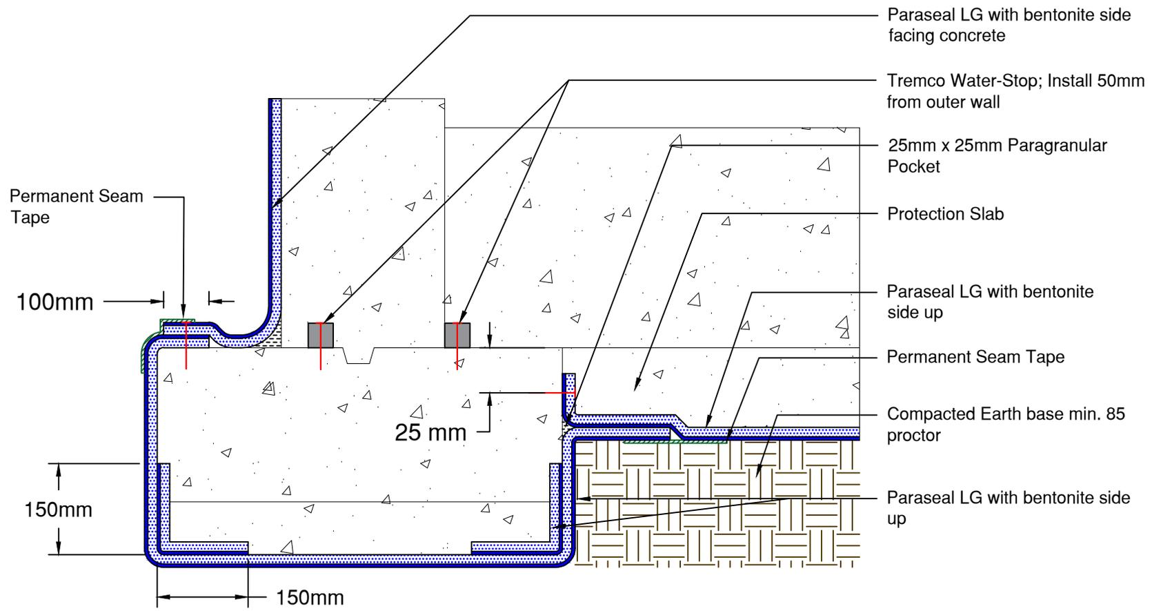
NOTE: Paraseal products require a min of 117jg/m2 of compaction/confinement in order to function as designed.
