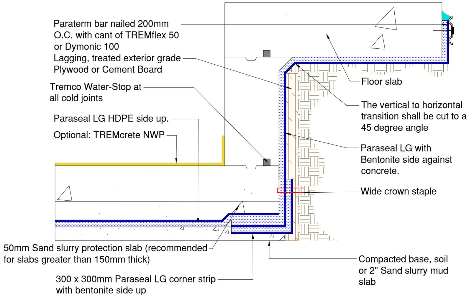
NOTE: Paraseal products require a min of 117Kg/m2 of compaction/confinement in order to function as designed.
