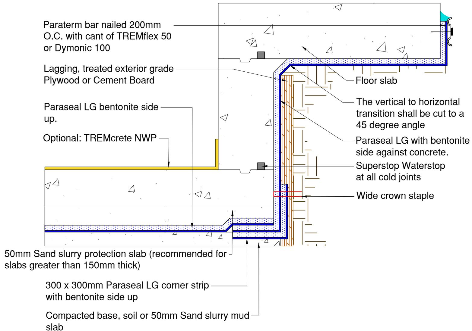
**NOTE:** Paraseal products require a min of 117Kg/m2 of compaction/confinement in order to function as designed.
