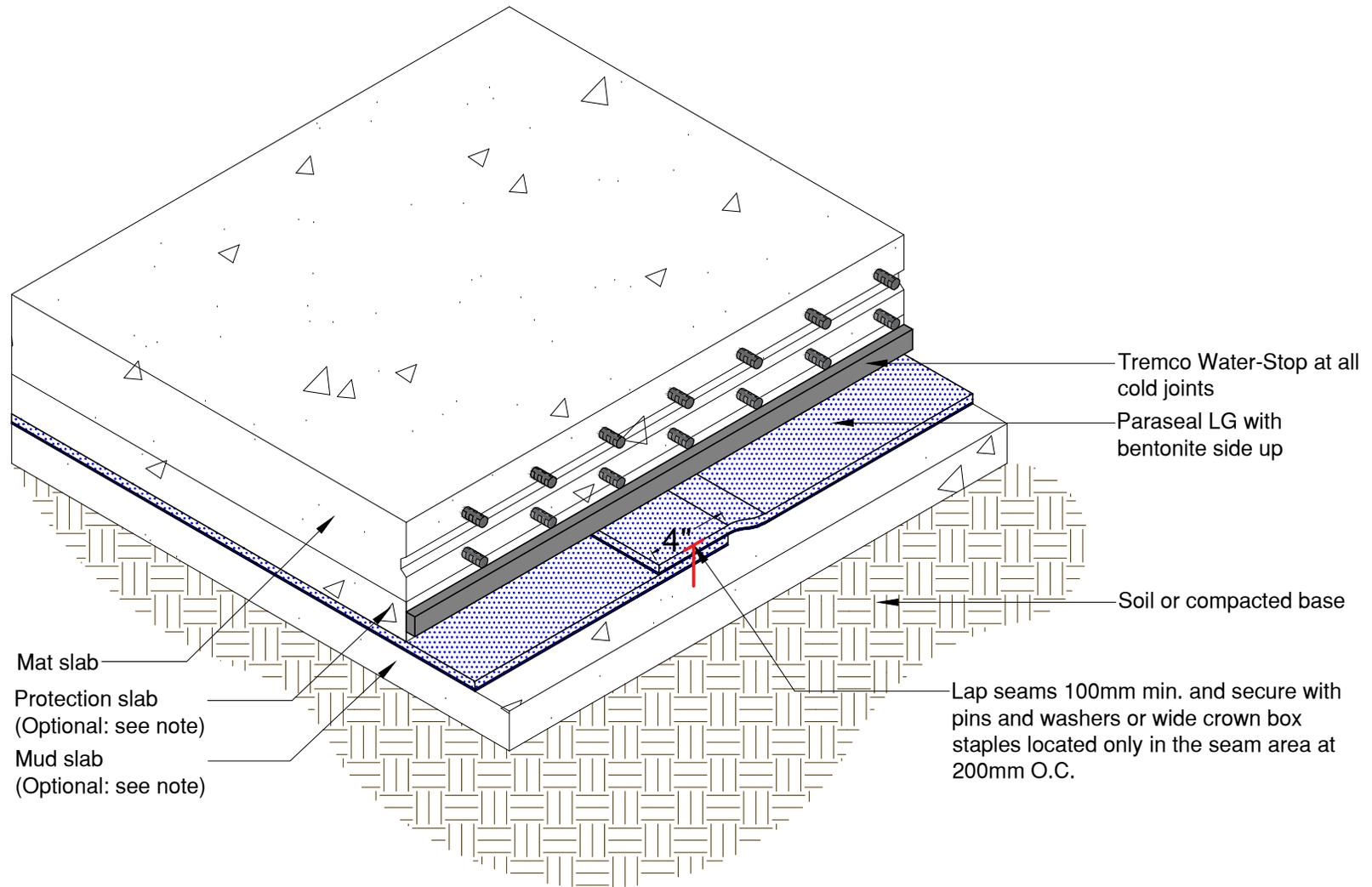
NOTE: Sand slurry protection slab and mud slab are recommended for heavily reinforced slabs greater than 150mm thick
