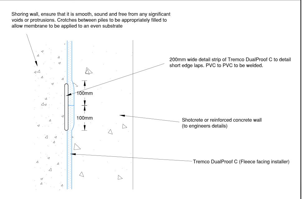
Note: Ensure that short edge laps are staggered by at least 300mm. Penetrations through short edge laps are not acceptable.
