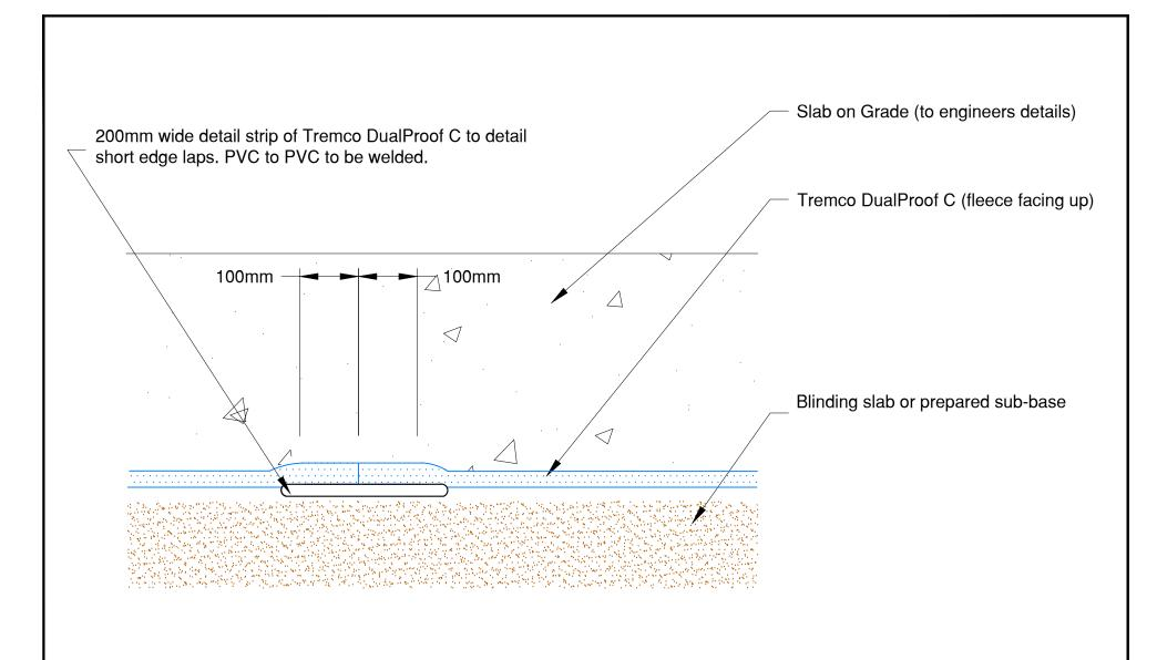
Note: Ensure that short edge laps are staggered by at least 300mm
