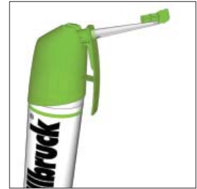
Figure 6: To store for future use push safety catch into nozzle end after use.
