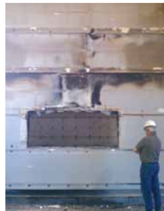
As the assemblies are dissected after the test, the extent of damage is exposed. In this case, though the aluminum skin started to peel away and the plastic core started to ignite, damage was contained to areas directly above the window and the assembly passed the test.
